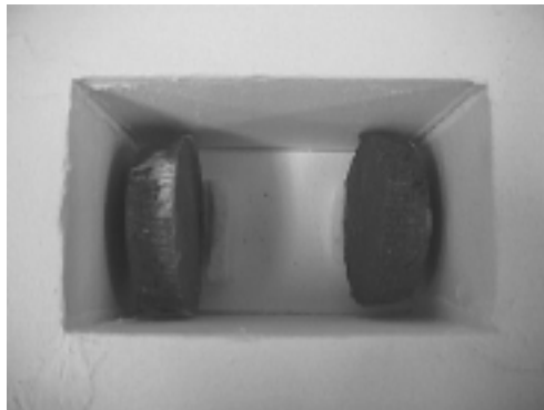
Figure 2. SiC susceptor placement inside insulation box (top view).
