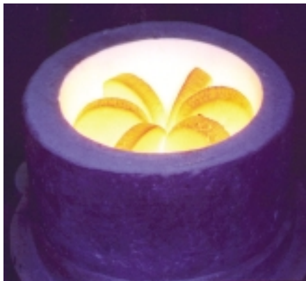
Silicon carbide discs in a microwave furnace.
