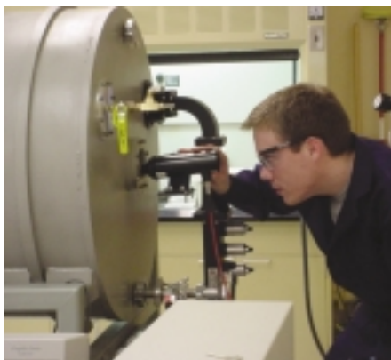
Jeff Miller, Ceralink engineer, peers through an optical pyrometer as materials heat up in the microwave.
