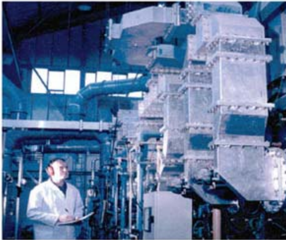
Fig 5 C-Tech Innovations (formerly EA Technologies) gas-assisted microwave firing systems; period kiln (top) and tunnel kiln (bottom)
