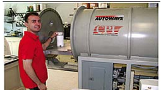
Fig 3 The CPI Autowave station can be fitted with different frequencies (2.45, 18 and 28 GHz) and power levels.
