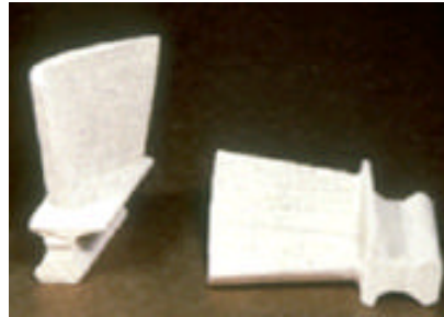
Figure 1. Green Silicon Nitride Turbine Blade Fabricated by the CerLAM Method
