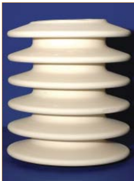
Fig. 4 Example of a Lapp insulator sample that was fired in a lab-scale MAT furnace at ~10 times the conventional firing rate.
