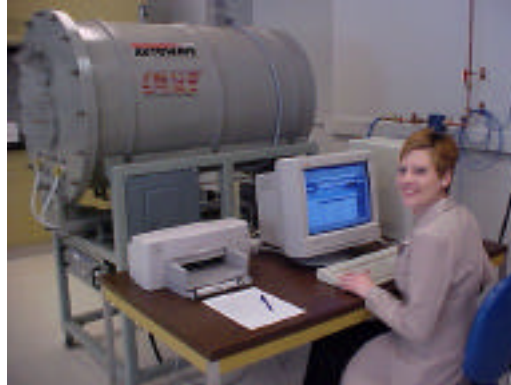
Figure 2. The CPI Autowave station can be fitted with different frequency (2.45, 18, 28 GHz) and power levels.
