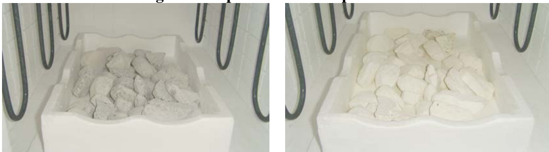
A) One kilogram of limestone in the mullite sagger in the MAT kiln A) pre-calcining and B) post calcining. Note the white color in B) indicating the product has been calcined.
