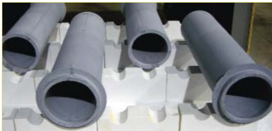
Fig. 3 Blasch SiC sleeves fired in a 30 ft 3 MAT electric kiln. These parts were successfully fired five times faster than Blasch's conventional firing cycle.
