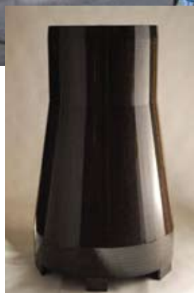
CFOAM composite tool for missile body application.
