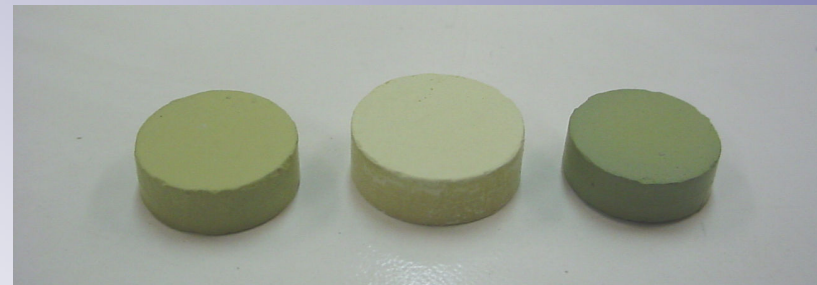
Figure 3. Contrasts the difference between conventionally sintered (A), green (B) and microwave sintered (C) pellets for 4% Sn doped pellets at 1400 °C sintering temperature.
