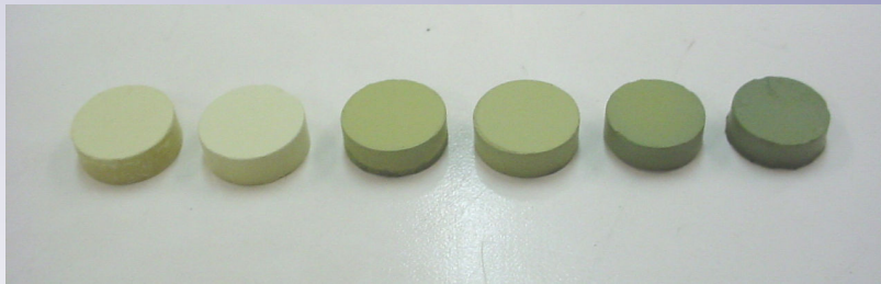
Figure 2. Various stages of pellet densification. These samples are 10% Sn doped and the sintering temperatures range from 1100-1500 °C. A color change is observed with the densification of indium oxide.
